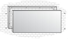
**Step 2**Slip sign panel over frame and secure with counter sink screws around perimeter.
